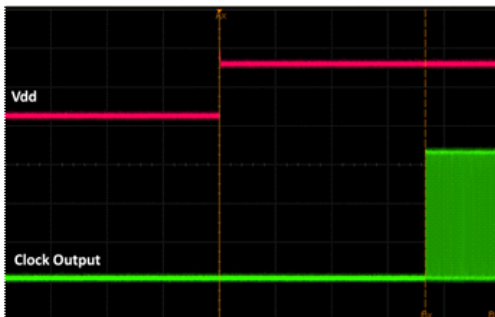
Figure 17. Startup Waveform vs. Vdd
